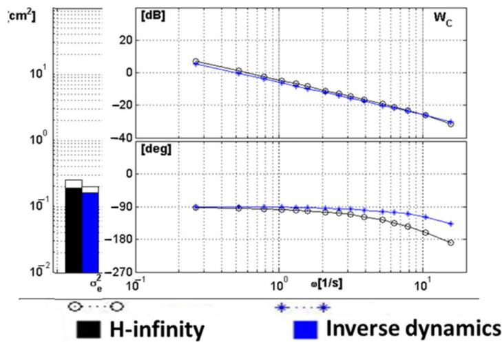
Figure 10. Inverse dynamics vs. H-infinity with actuator constraints and high gain.
