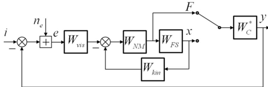
Figure 6. Modified pilot structural model.
