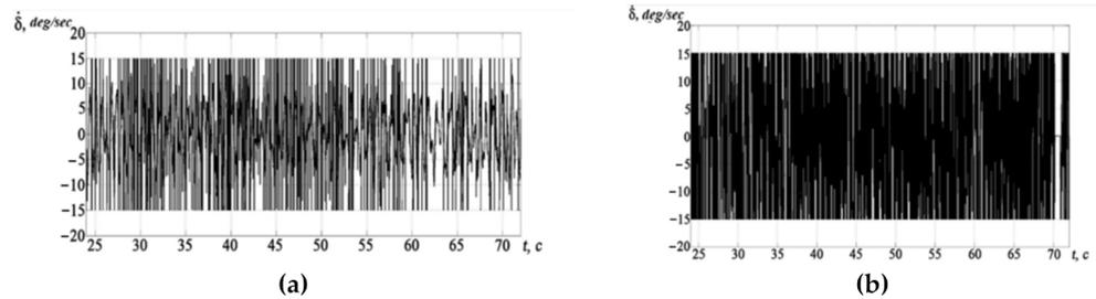
Figure 17. Rate  $\dot{\delta}(t)$  of the control signal. (a) DSC, (b) FSC.
