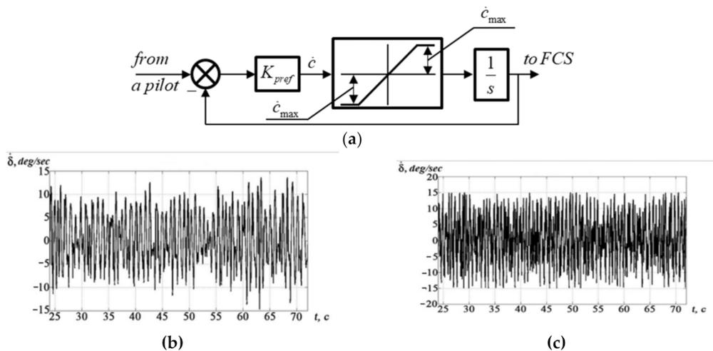
Figure 18. Effect of a non-linear prefilter. (a) function demonstration of nonlinear prefilter, (b) DSC, (c) FSC.
