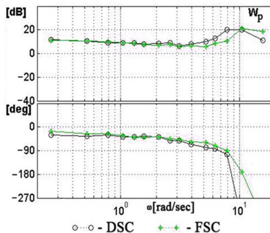
Figure 15. Pilot describing functions for DSC and FSC pilot output.
